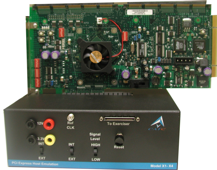
Host emulation test fixture with DUT card on top
